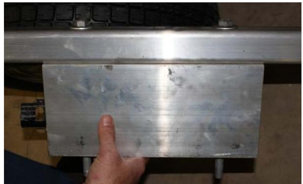
3- Place the "Axle Spacer" on top of the mounting plate on the axle with the bolts going through the holes on the axle mounting plate. Attach using one (1) 1/2" galvanized washer, one (1) 1/2" galvanized lock washer and one (1) 1/2" galvanized nut on each bolt.
