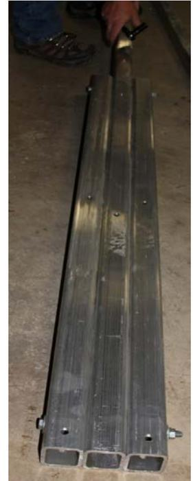
3- Next lay the "Tongue Tube" onto the bucket. When doing so, put it down so the vin number is on the side and in an upright position as if you were going to read it. You should position the bucket so it is between the two holes. (If you are doing the assembly by yourself you may want to keep the "Tongue Tube" on the ground to keep the parts from falling off of the bucket).
