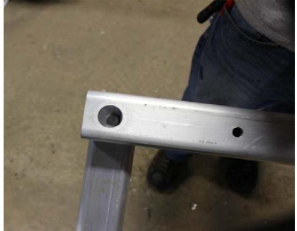
Attach the "Short Cross Tube" to the "Side Tube" using one (1) 3/8 galvanized washer, one (1) 3/8 galvanized lock washer and one (1) 3/8" nut in each hole. Hand tighten only.
