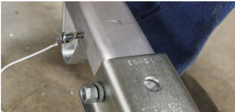
13- Using the remainder of the Wire Loom, start at the end of the wires where the plug is. Push all of the wires into the wire loom. At some point the white ground wire will have to come out of the Wire Loom and you will continue pushing the other wires into the Wire Loom. The Wire Loom will need to cover the wires going into the "Tongue Tube" at least two (2) inches. You can cut any remaining of the Wire Loom off.
