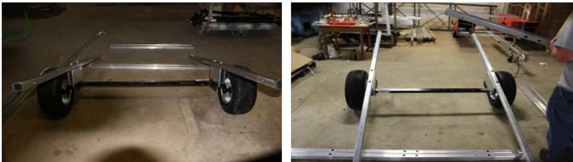
5- Take one (1) of the "Short Cross Tubes" and attach it to the front of the "Side Tube" using one (1) of the 3/8 - 16 x 3" galvanized bolts on each side. The "Short Cross Tube" has larger holes on one side vs. the other side. The larger holes will go up ↑. Insert the 3/8 - 16 x 3" galvanized bolt through the larger hole and into the smaller hole on the other side. Then put the bolt through the hole on the top of the "Side Tube" inserting it all the way through the "Side Tube."
