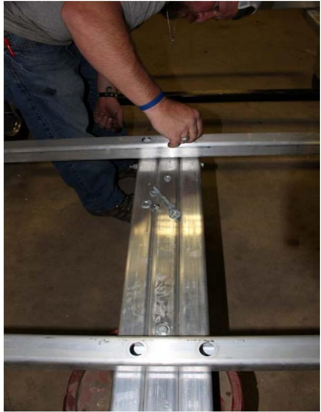
2- Line up the holes on the "Long Cross Tube" and the holes on the "Short Cross Tube" with the holes on the Tongue Assembly.
