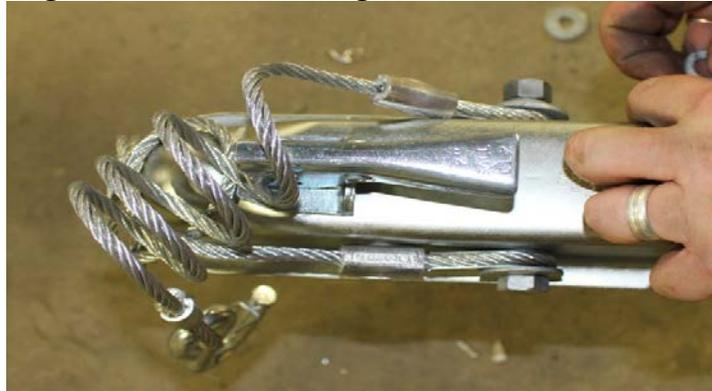
5- Take the 1/2-13 x 3" galvanized bolt and insert it through the other hole in the Coupler going through the "Tongue Tube." Secure this with one (1) 1/2" galvanized lock washer and one (1) 1/2" galvanized nut and tighten.
