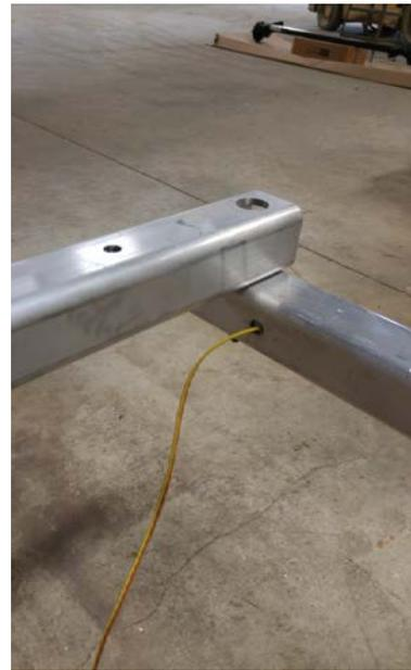
3- Push the tape measure all the way through the "side tube" from the rear. Tape the wires onto the tape measure and pull the wires back through the "Side Tube."
