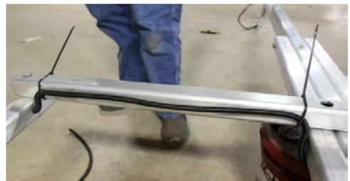
Pinch the Wire Loom so one side of it folds into the other making it a smaller circle and push this into the hole in the side of the "Side Tube" so the Wire Loom protects the wire into the hole.
