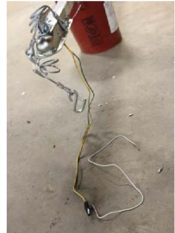
2- Take the yellow & brown wires and pull it to the left side of the trailer, take the green/brown wire and put it on the right side of the trailer. The "sides" are determined by looking to the front of the trailer from the back.
